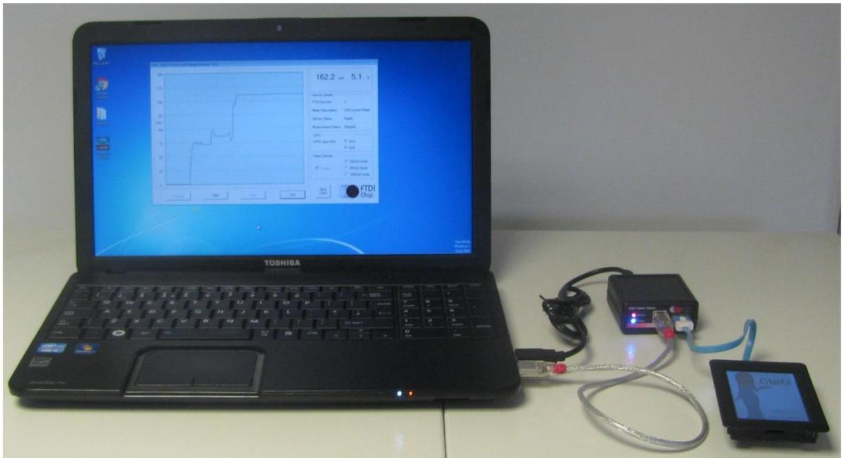
**Figure 11 – Connecting the unit to measure the current consumed by a CleO board**
